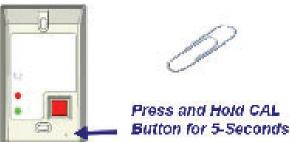
e. Verify the alarm set point is calibrated properly by modulating the exhaust volume or moving the fume hood sash to achieve the desired alarm set point.
